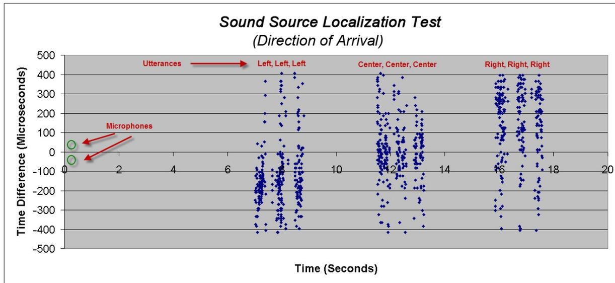
This was a simple test but it can be seen that the grouping of the WIVs correlates well with the speaker's position in the room. Localization could have improved by using a more robust mathematical algorithm and by reducing sound reflections within the room.
